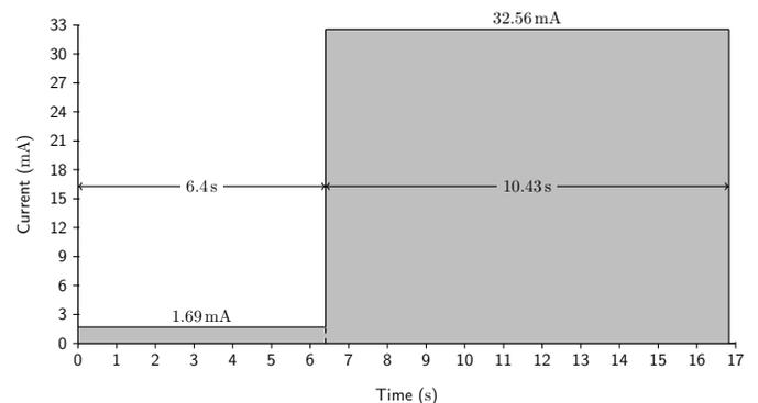
Fig. 2: Current consumption as a function of time for Configuration 1 (sample and transmit raw data).
