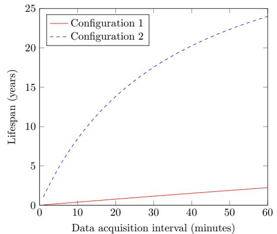
Fig. 4: Theoretical lifespan of the tags for various data acquisition intervals. Calculations are based on a 3.7 V (1800 mAh) lithium-ion battery.
