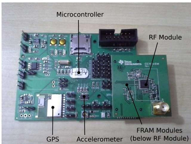
Fig. 1: Assembled biotelemetry tag. The tag measures 100 mm x 60 mm x 12 mm and weighs 32 g.
