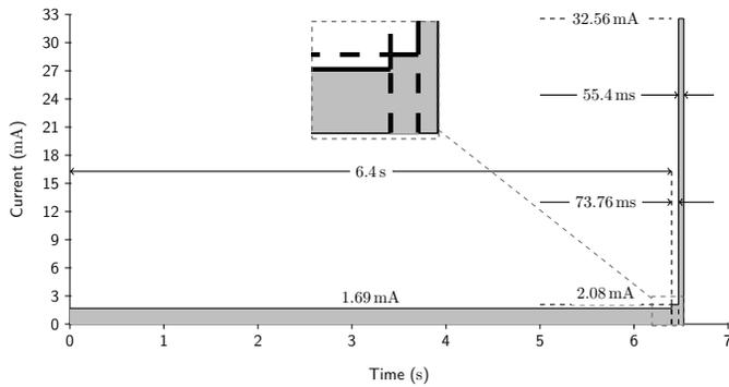
Fig. 3: Current consumption as a function of time for Configuration 2 (sample, classify and transmit decision).
